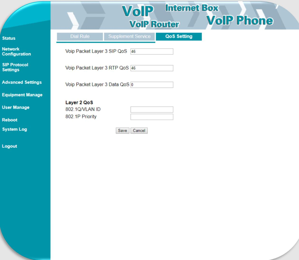
The screenshot shows the web interface for a VoIP Router. The main header reads "VoIP Internet Box VoIP Router VoIP Phone". Below the header are three tabs: "Dial Rule", "Supplement Service", and "QoS Setting" (which is selected). The "QoS Setting" page contains the following configuration fields:
